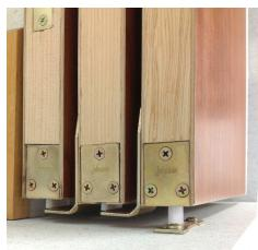
Side mount guide posts can be used to allow for a setup that does not require bottom guide tracks. Individual guide posts are used and .052 6063T6 Aluminum track, 14-16 gauge steel parts travel inside a groove in the bottom of each door to make for a clean floor in the opening.
